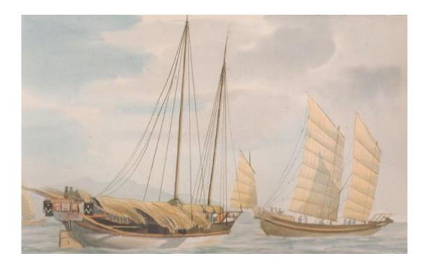
51: Passage boat from Macao to Canton. Length 50 to 65 feet; Width 10 to 12 feet; Hull 7 to 8 feet.
